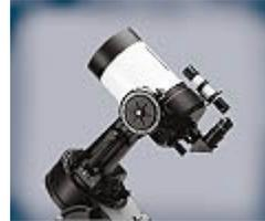
Alternatively, short-focus refractors are available in 2.7- to 3.1-inch (70- to 80-mm) apertures with tubes short enough to fit into a camera case. Primarily designed for low-power, wide-field views of the stars, these refractors also work well for moderate-power views of the planets. All require a sturdy tripod at extra cost.
