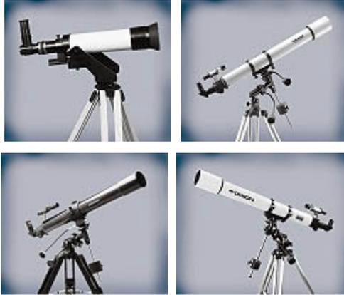
Above: Many companies sell small refractors on altitude-azimuth or equatorial mounts, including (from upper left) Tele Vue, Meade, Celestron, and Orion. The higher the optical quality and the sturdier the mount, the happier you'll be with your purchase -- *especially* for such small-aperture instruments.
